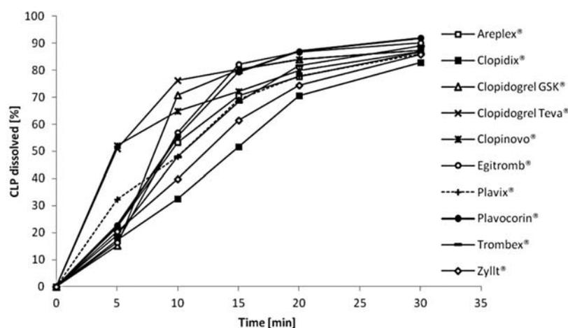
Figure 3. Mean dissolution profiles (n = 6) of ten CLP 75 mg products (apparatus 2, 50 rpm, 1000 mL of pH 2.0 hydrochloric acid buffer, first stage ( $S_1$ ) of the dissolution test, CLP determined using CE assay)
