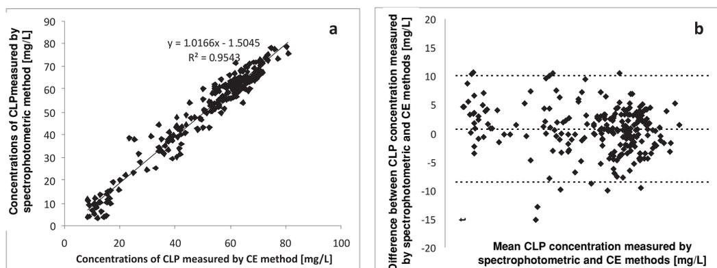
Figure 2. Plots for the Bland-Altman analysis. a – scatter plot of the CLP concentrations determined by UV spectrophotometric method versus those obtained by CE method; b – Bland-Altman plot of the difference between the CLP concentrations determined by UV spectrophotometric and CE methods against the mean of the concentrations
