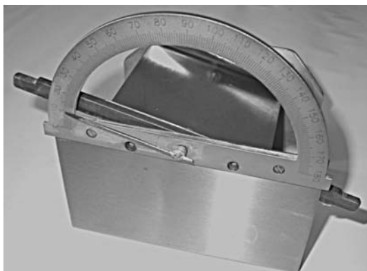
Figure 1. Equipment for the evaluation of angle of slide
